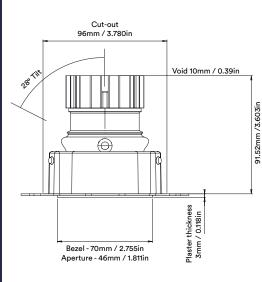
Unit height increases by 21.65mm / 0.85in for spot and elliptical beams
