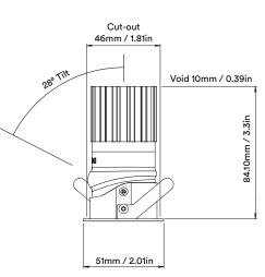
Unit height increases by 12mm / 0.48in for SPOT and both ELLIPTICAL BEAMS
