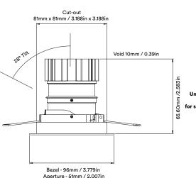
Unit height increases by 21.65mm / 0.85in for spot and elliptical beams
