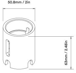
Optional Installation sleeve for screeding and masonry applications only
