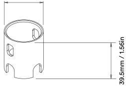
Optional Installation sleeve for screeding and masonry applications only
